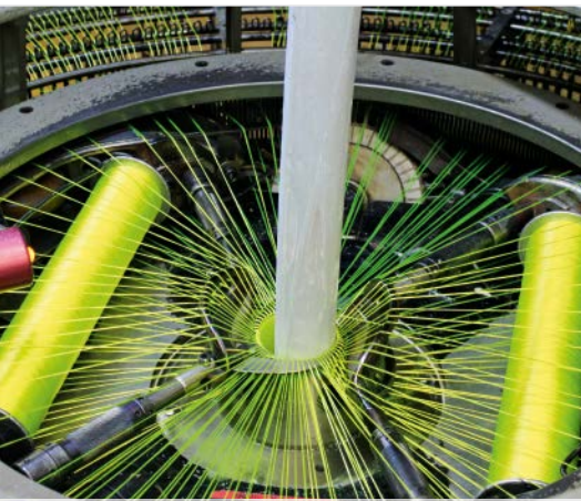
weaving process of jacket with incoming rubberlining
